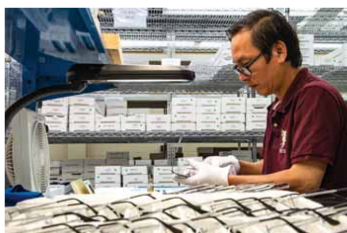
A worker adds lenses and puts the final assembly touches on the 200-step process to complete a single pair of sunglasses, before being boxed and shipped.
