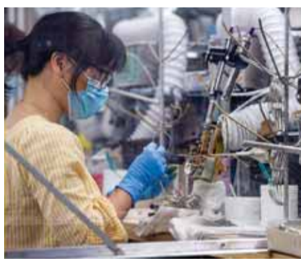
A worker solders the frame and other components of the sunglasses as part of the 200 steps required to complete a single pair, with the entire build taking six weeks.
