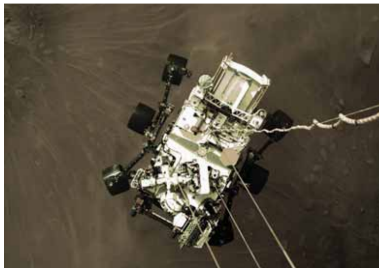
This photo released by NASA shows the Perseverance rover being lowered by the Sky Crane to the surface of Mars on Feb 18, 2021. — AFP photos
