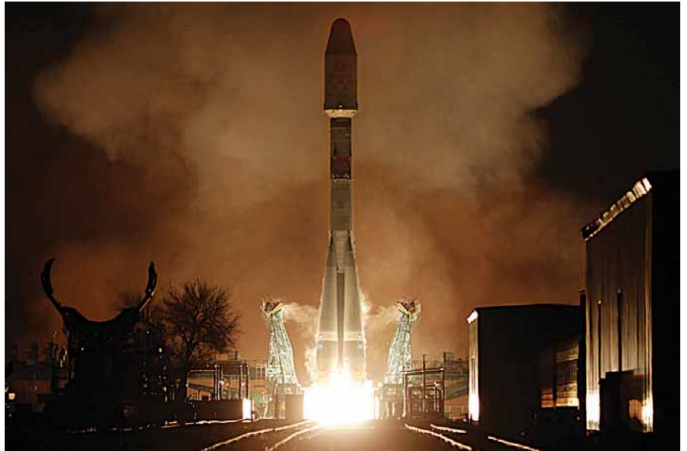
Photo shows a Soyuz-2.1b rocket booster with a Fregat upper stage and satellites of British firm OneWeb blasting off from a launchpad at the Baikonur Cosmodrome.
