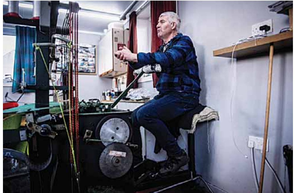
Harris tweed weaver Ian Mackay works on his pedal powered loom.
