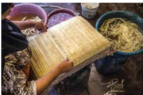
A woman lays out soaked thin strips of papyrus to form a sheet, before compression and drying at the workshop in the village of Al-Qaramous.
