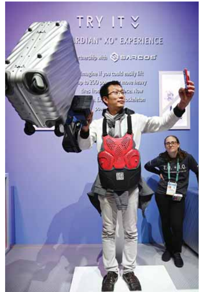
An attendee takes a selfie as he lifts a 50 lb (22.7 kg) suitcase with the help of the Sarcos Guardian XO exoskeleton arm on Wednesday at the 2020 Consumer Electronics Show (CES) in Las Vegas.
