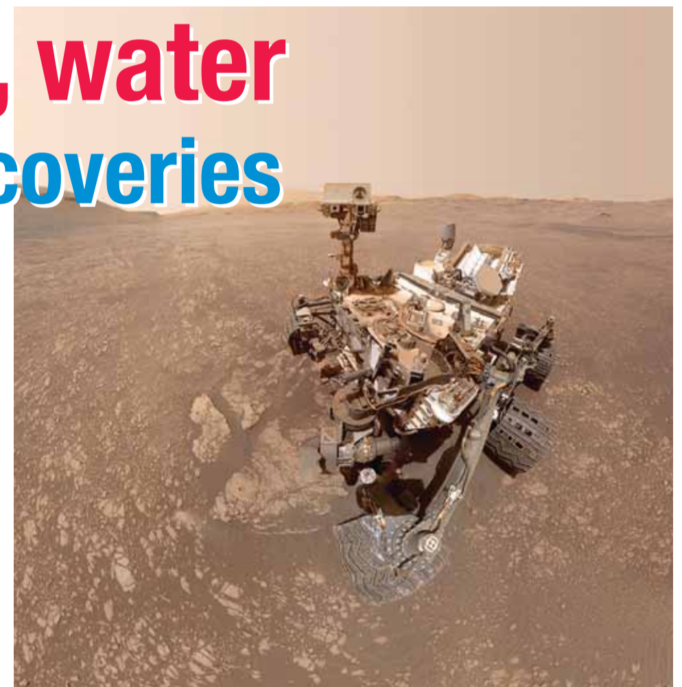
In this image obtained from NASA, the Curiosity Mars rover took this selfie on May 12, 2019 (the 2,405th Martian day, or sol, of the mission). To the lower-left of the rover are its two recent drill holes, at targets called "Aberlady" and "Kilmorie".
