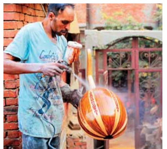
A man sprays varnish on an Arabian Oud at a workshop belonging to Khaled Azzouz.
