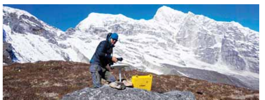
A Nepal Survey Department team member places a Global Navigation Satellite System (GNSS) receiver after drilling it on a rock during Mount Everest's height measurements. — AFP
