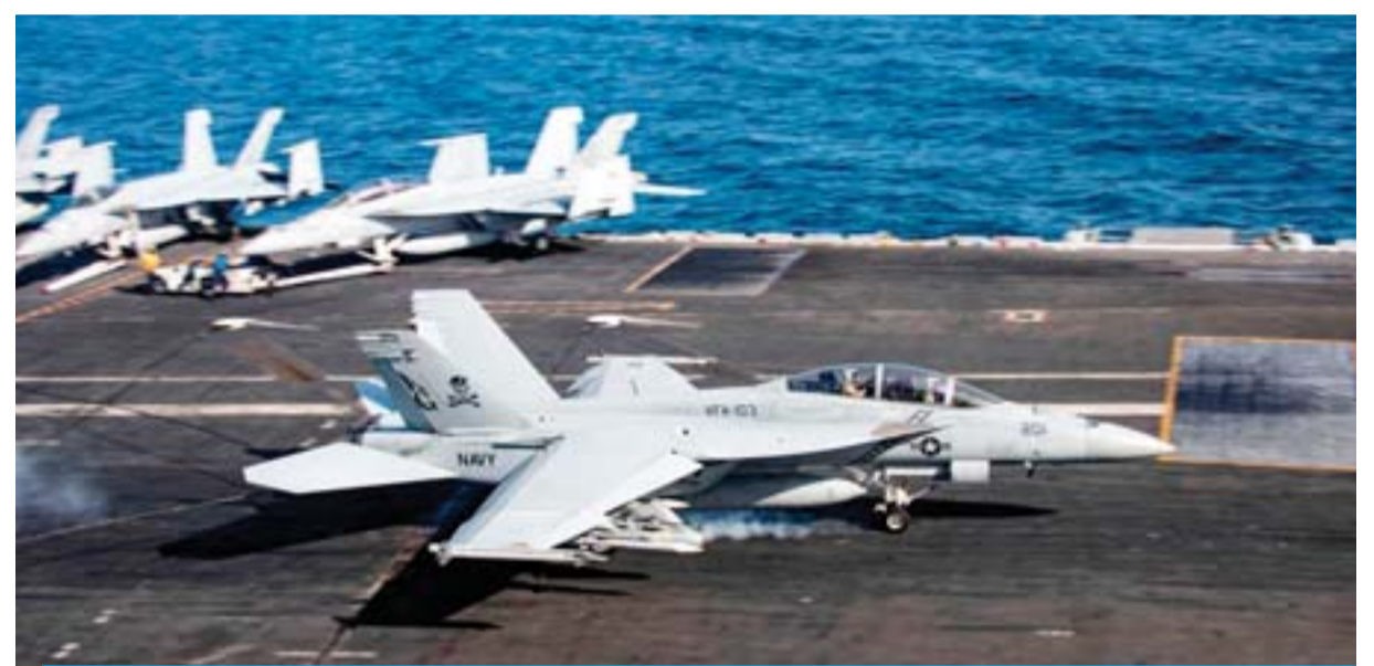
AT SEA: Photo shows an F/A-18F Super Hornet from the 'Jolly Rogers' of Strike Fighter Squadron (VFA) 103 making an arrested landing on the flight deck of the Nimitz-class aircraft carrier USS Abraham Lincoln (CVN 72) in the Gulf of Oman. - AFP
