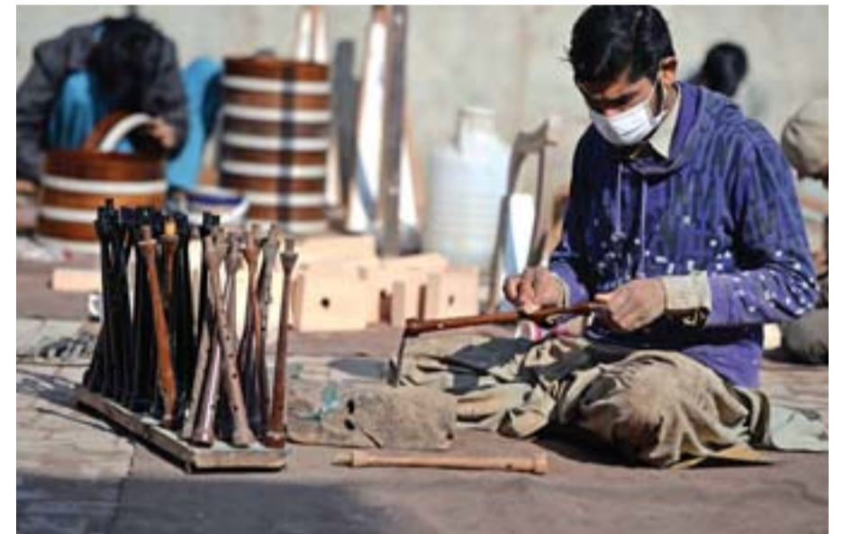
A Pakistani worker polishes a component to be used to make a set of bagpipes at the Mid East bagpipe factory in the eastern city of Sialkot.
