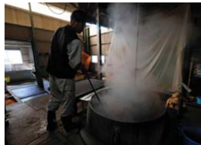
A worker boiling kozo plants at the beginning of the papermaking process.
