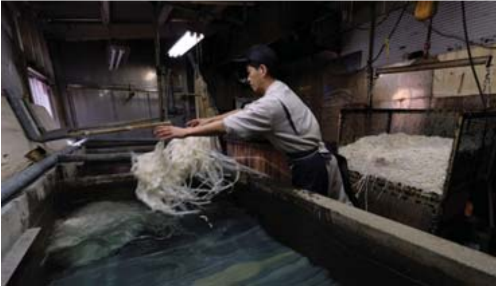
Worker putting steamed kozo plants in a water tank during the “washi” paper manufacturing process at the Hidaka Washi factory in Hidaka, Kochi prefecture. — AFP photos
