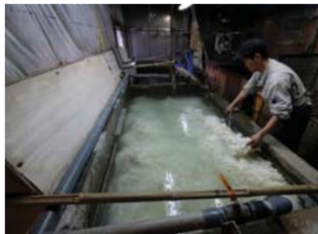
A worker putting steamed kozo plants in a water tank during the “washi” paper manufacturing process.
