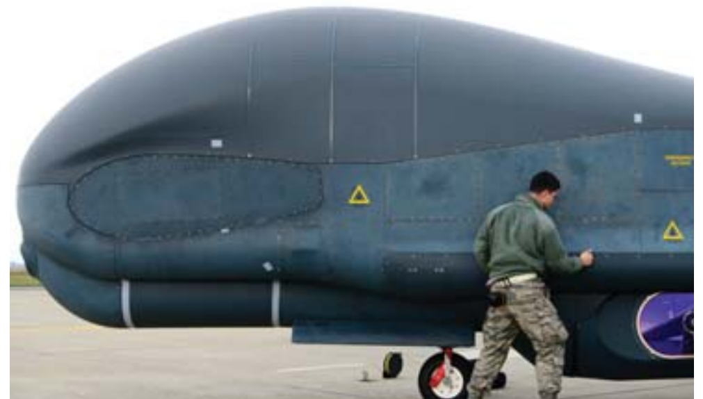
In this image released by the US Air Force, Staff Sgt. Seth Thurber checks panels of a RQ-4 Global Hawk unmanned surveillance drone during a preflight inspection, at Beale Air Force Base, California. — AFP
