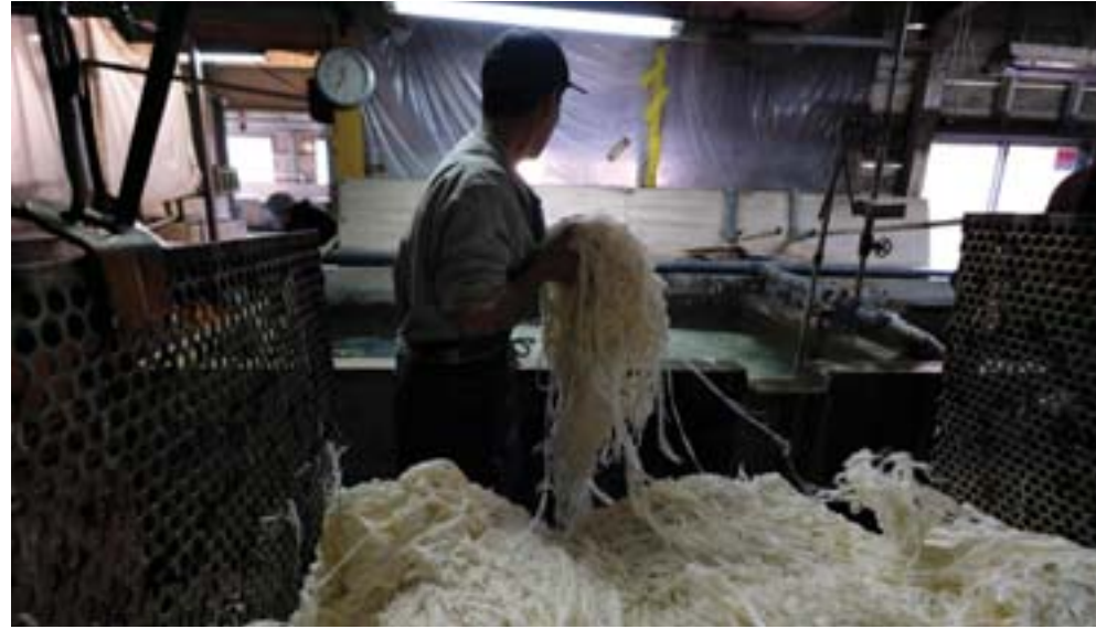
Worker putting steamed kozo plants in a water tank during the “washi” paper manufacturing process at the Hidaka Washi factory in Hidaka, Kochi prefecture. — AFP photos
