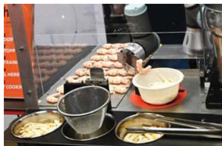
A robotic chef named Sophie prepares a bowl of laksa, a local dish of rice noodle in curry sauce.
