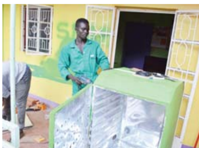
Affordable machine to dry fruit and vegetables helps farmers stop harvests spoiling and burns green briquettes, not charcoal, for heat.
