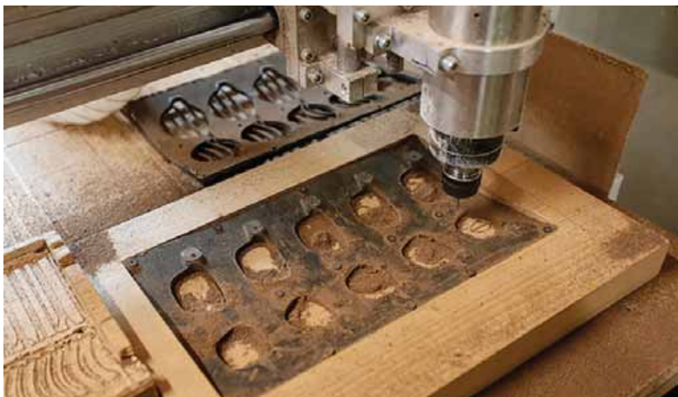
A cutter makes eco-friendly sunglass frames from coffee waste.
