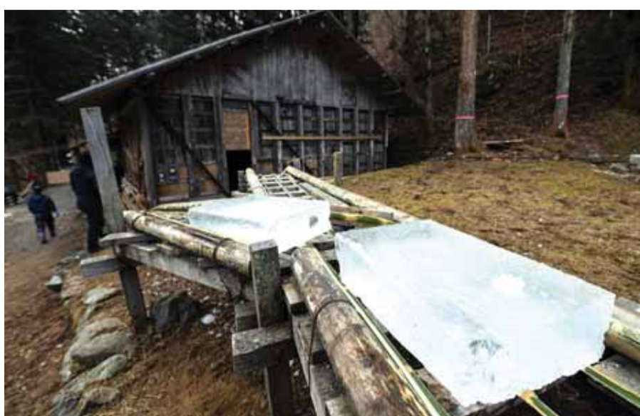
Blocks of natural ice being moved on a bamboo rail after being cut from an open-air pool at a factory in Nikko, Tochigi prefecture.
