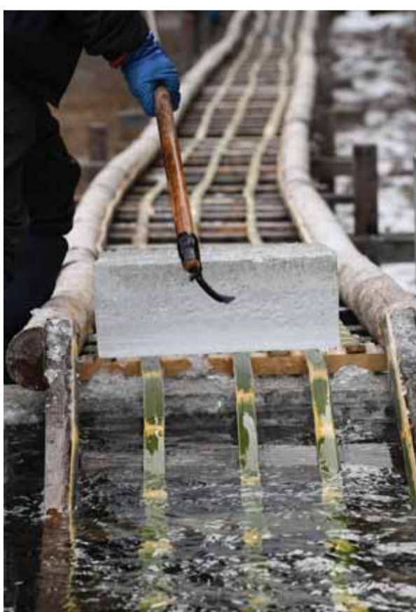
A worker sliding a block of natural ice on a bamboo rail after it was cut from an open-air pool at a factory in Nikko.
