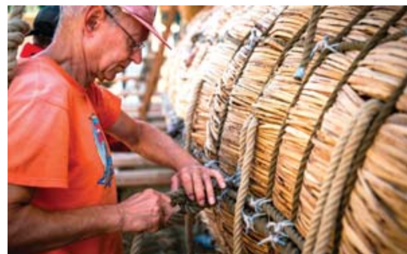
A member of the crew assembles the 14-meter long sailing reed boat Abora IV.
