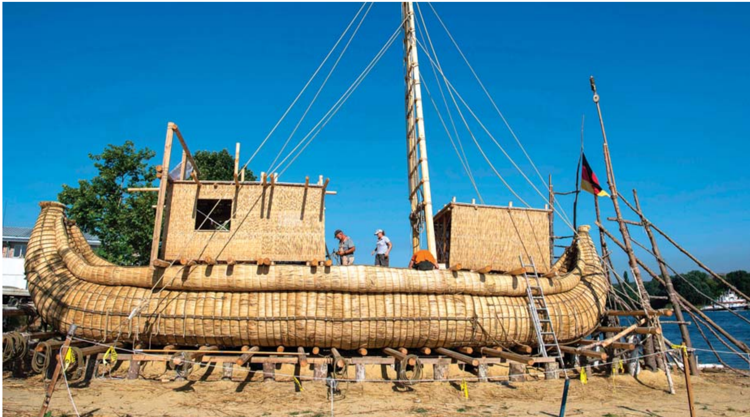
Members of the crew assemble the 14-meter long sailing reed boat Abora IV in the town of Beloslav, Bulgaria.— AFP photos
