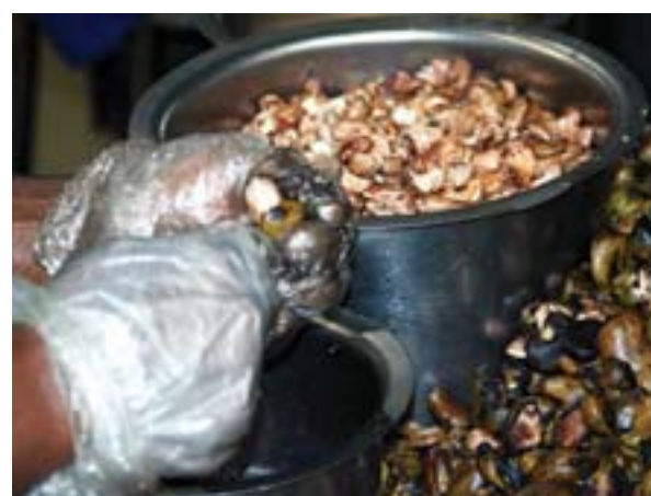
A Fludor factory worker removes a cashew nut's almond with a knife at the Fludor plant.
