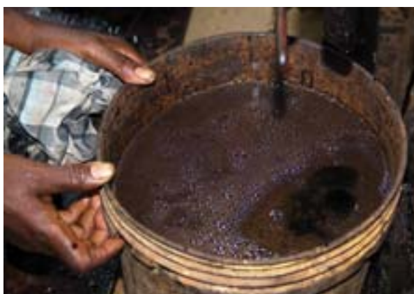
A worker collects cashew oil, or cashew nut shell liquid (CNSL), extracted from the nuts' crushed shells at the Fludor plant.
