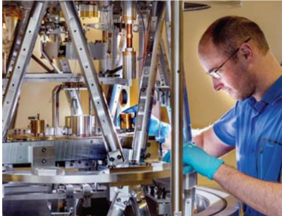
SEVRES, France: A handout photo taken in 2018 and made available yesterday shows a scientist at work on the kibble balance, an electromechanical weight measuring instrument that measures the weight of a test object very precisely by the strength of an electric current and voltage. — AFP
