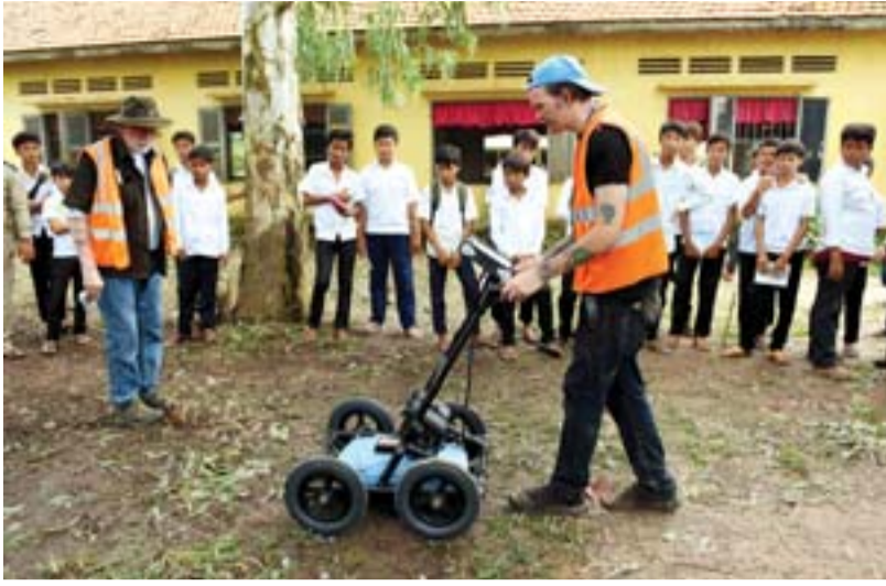
This photo shows David MacMillan, an expert from SparrowHawk Far East company, operating the ground-penetrating radar machine while students look on during a search for mass graves at a school compound in Prey Veng province.
