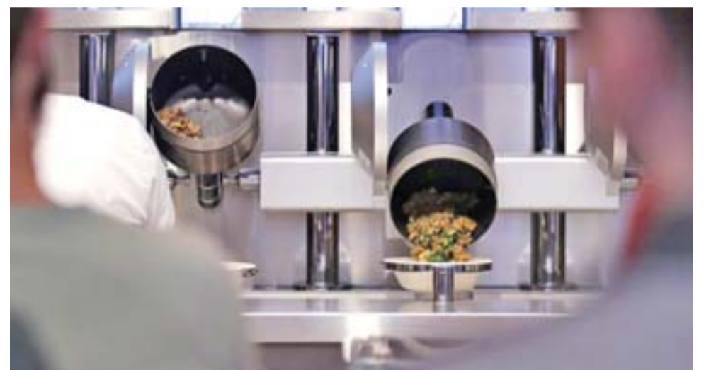
Customer wait as their automatically prepared food is dropped from a cooking pot into a bowl at Spycy, a restaurant which uses a robotic cooking process.
