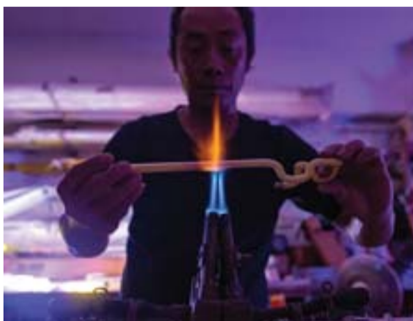
Wu Chi-kai demonstrates how to make a neon sign.
