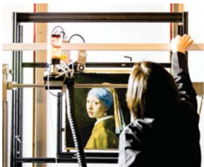
This picture shows Johannes Vermeer's "Girl with a Pearl Earring" painting inside a XRF macro-scanner during a research at Het Mauritshuis in The Hague. — AFP
