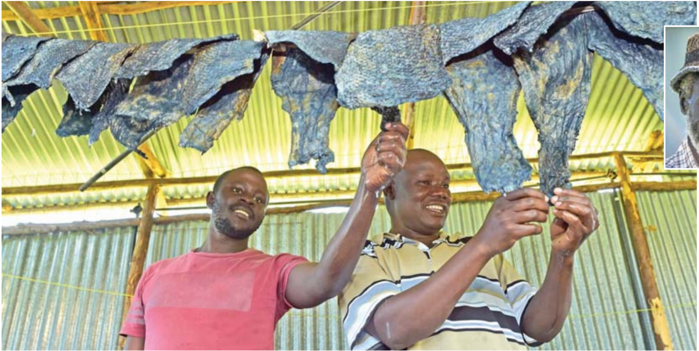
Newton Owino (right), an industrial chemist, hangs tanned fish pelts with the help of an employee after a soak in a softening formula concocted from extracts. — AFP photos
