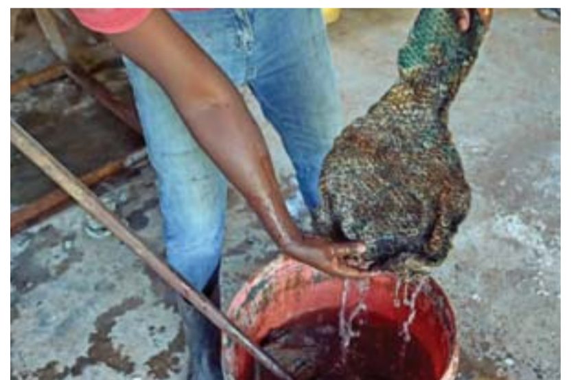
An employee soaks tanned fish pelt in a softening formula at the Alisam Product Development.
