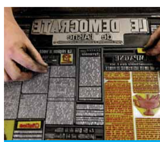
A worker adjusts letters on a plaque in the printing company's workshop of the "Democrate de l'Aisne".
