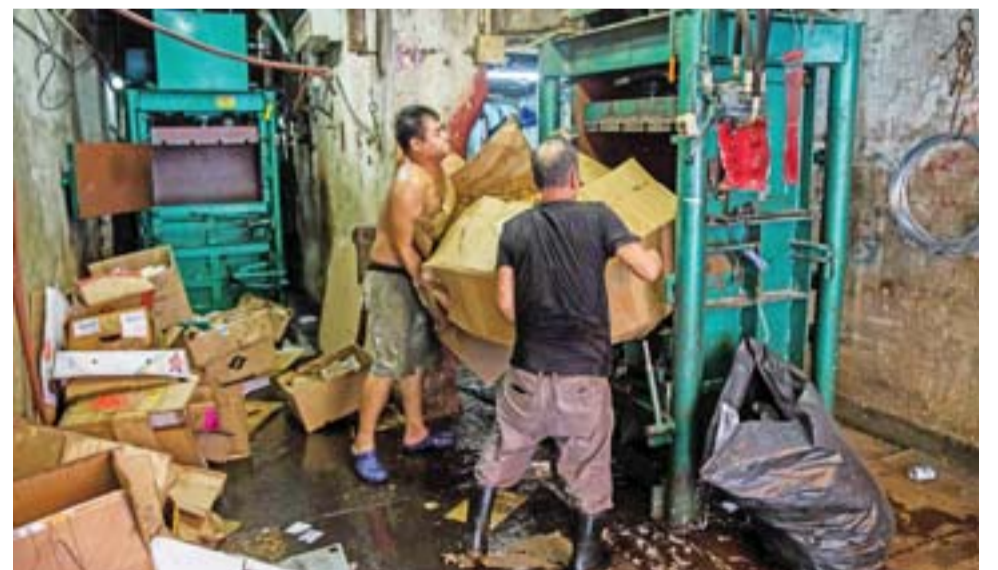
This picture shows workers at a recycling depot loading cardboard into an industrial compactor.
