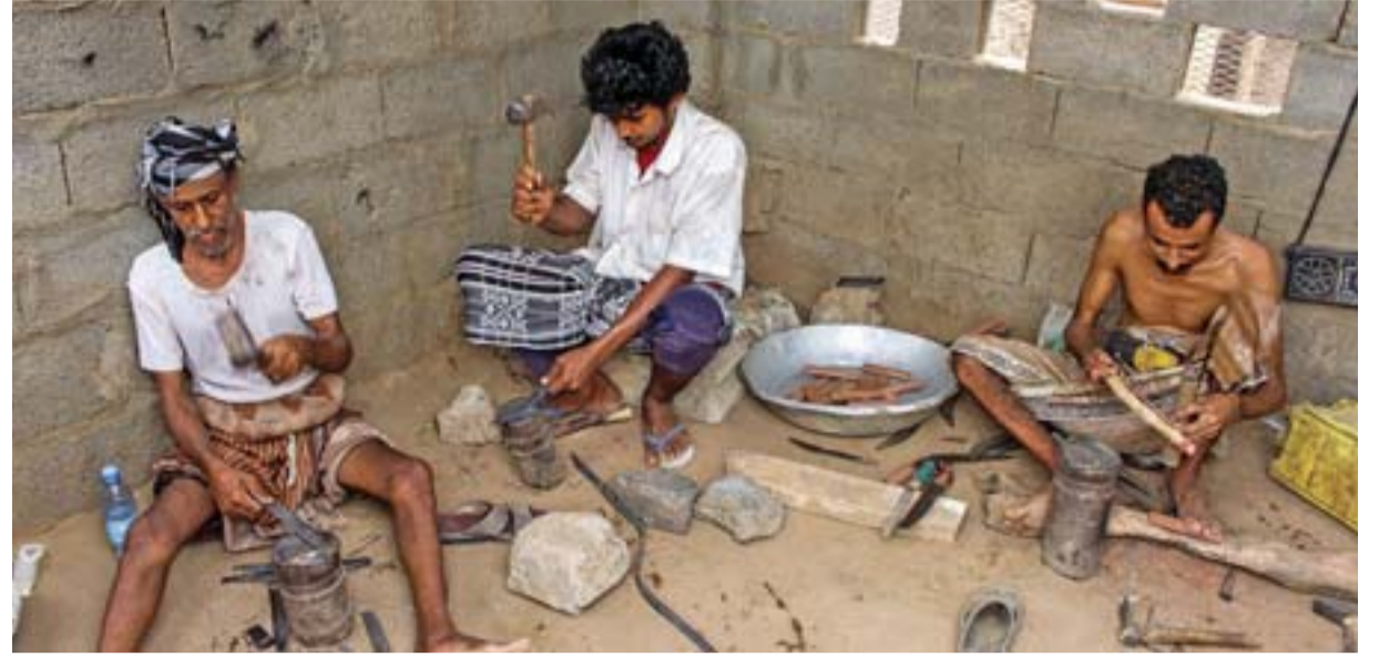
Yemenis hammer blades reformed from metal salvaged from fallen rockets in air strikes to create blades for new daggers.
