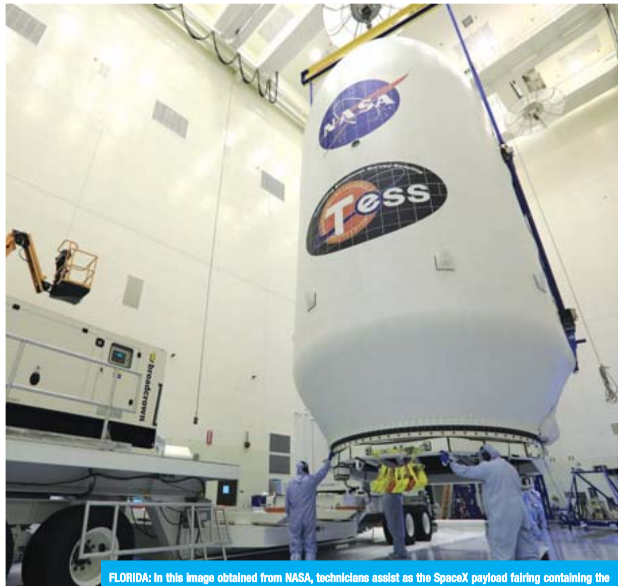
FLORIDA: In this image obtained from NASA, technicians assist as the SpaceX payload fairing containing the NASA's Transiting Exoplanet Survey Satellite (TESS) is moved by crane to a transporter inside the Payload Hazardous Servicing Facility at NASA's Kennedy Space Center, Florida.—AFP
