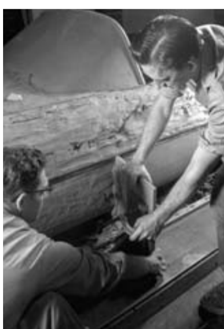
This 1954 photo Courtesy of General Motors shows Buick Design Studio creative clay sculptors as they mold the clay on a model GM automobile. — AP
