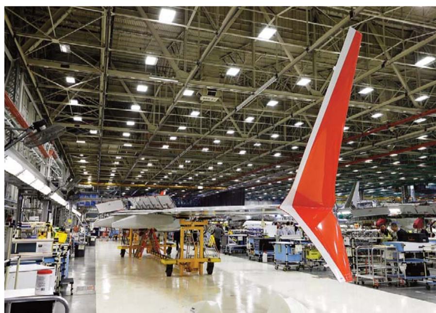
WASHINGTON: Boeing 737 MAX winglets, which sweep up and down from the wingtip and differ from the current 737 model with its single upward wingtip sweep, stand already painted in the Lion Air livery as the wing is assembled at Boeing's airplane production facility in Renton, Washington.—AP
