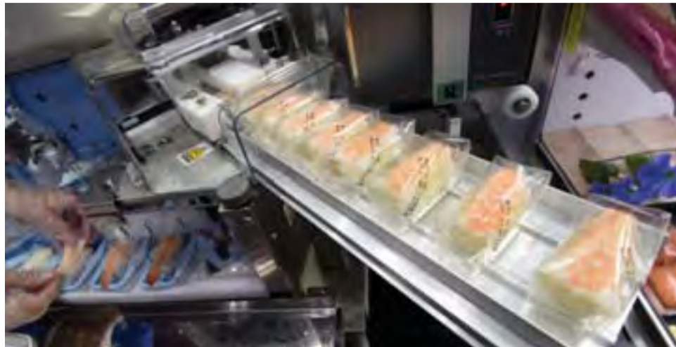
An employee of Japan's cooked rice processing machine maker SUZUMO demonstrates their automatic sushi wrapping machine at the International Food Machinery and Technology Exhibition in Tokyo. — AFP photos
