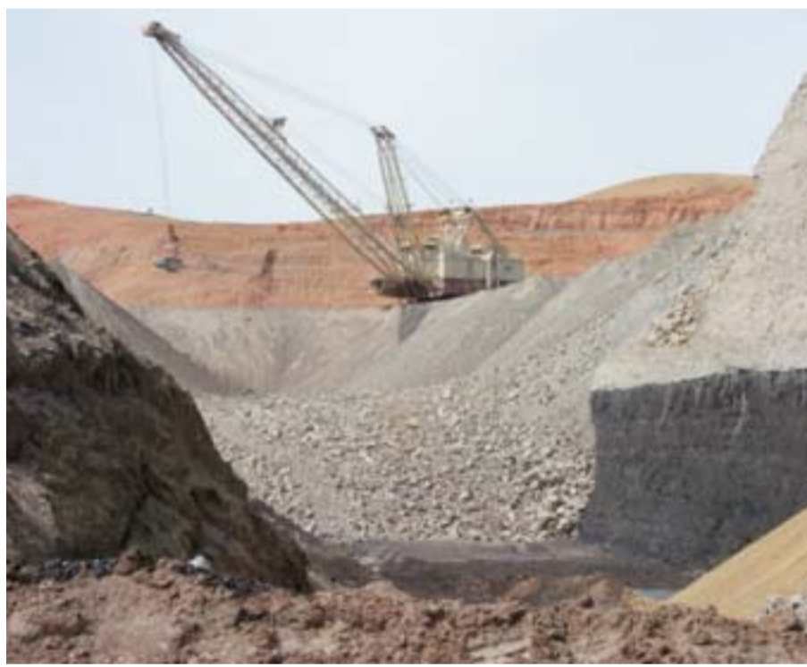
DECKER, Montana: In this April 4, 2013, file photo, a dragline excavator moves rocks above a coal seam at the Spring Creek Mine. — AP
