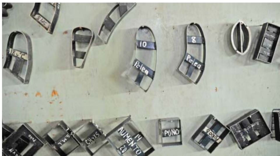
Iron molds used to produce different shapes and sizes of boxing gloves.
