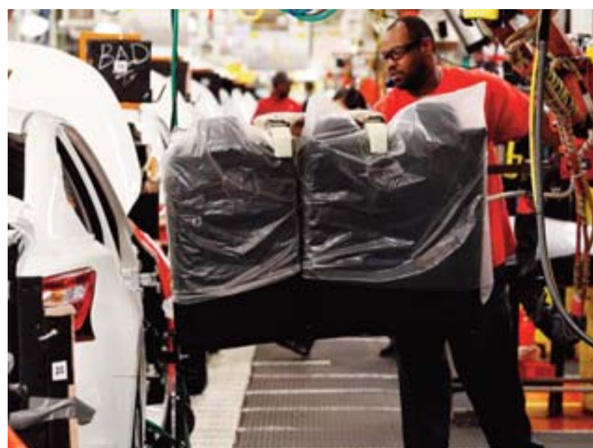
CANTON: In this April 6, 2016, photograph, a technician uses a lift to move a back seat section into a new Altima on the assembly line at the Nissan Canton Vehicle Assembly Plant. —AP
