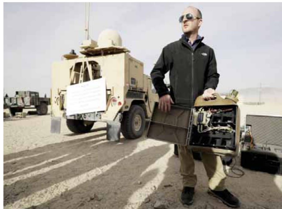
TWENTYNINE PALMS, California: In this Dec 7, 2016 photo, engineer Tyler Wagner displays batteries made to fit into a fuel container during an exhibition of green energy technology. — AP
