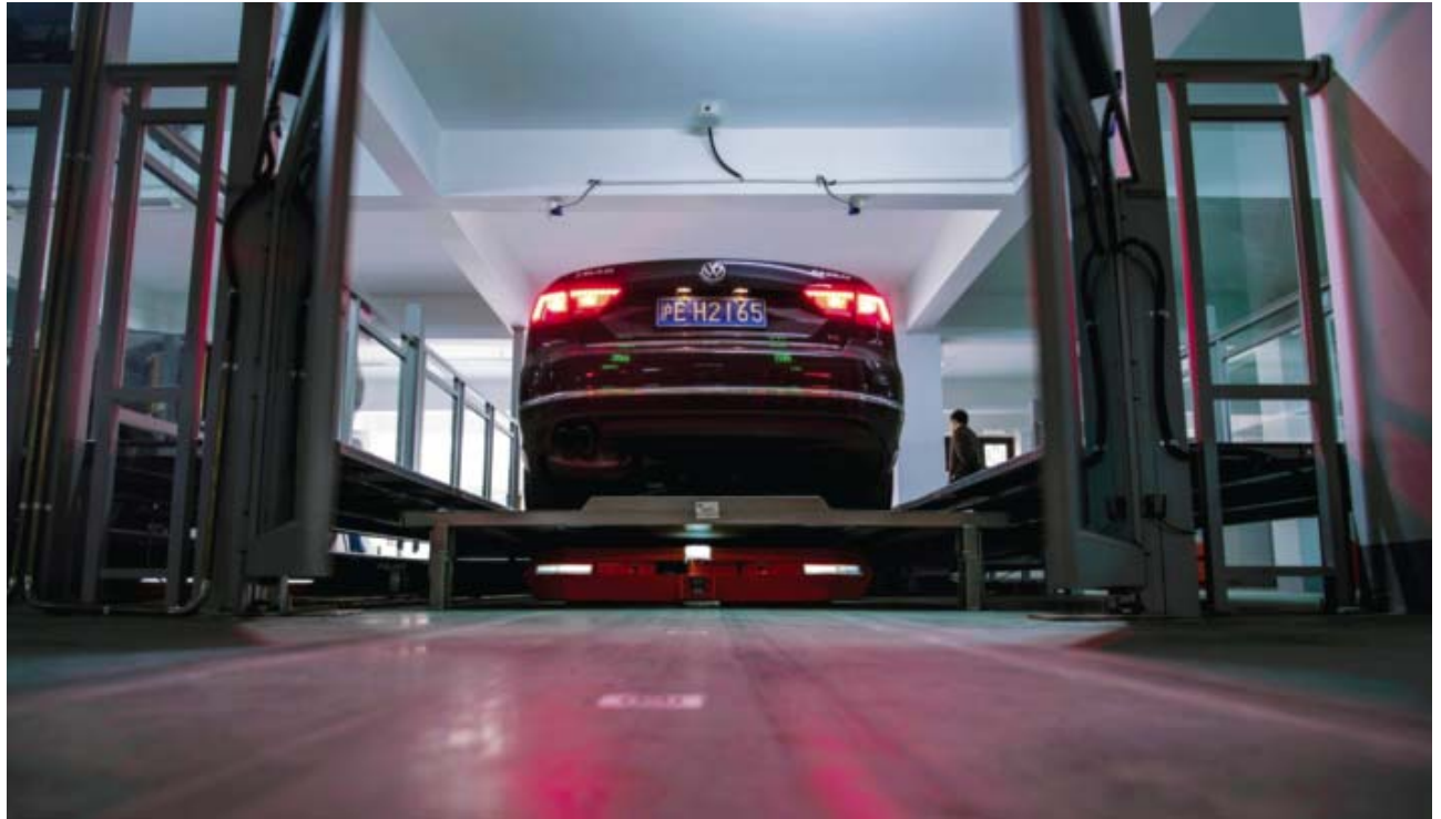
TONGXIANG CITY, China: This picture taken on Nov 25, 2016 shows people watching a robotic unit of the smart parking system developed by Hikvision in a garage in Wuzhen Township in east China's Zhejiang province.—AFP
