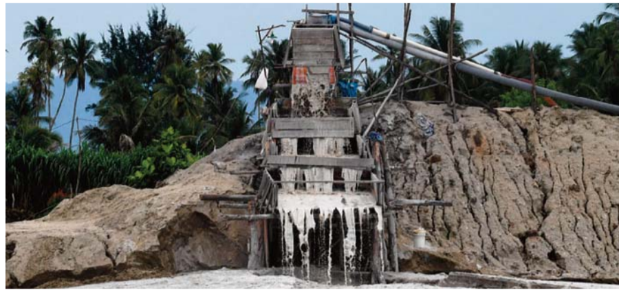
SUNGGAI LIAT, Indonesia: This photo shows a pump dredging sediment from a pit mine located inland from Sungai Liat.
