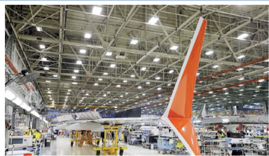
WASHINGTON: Boeing 737 MAX winglets, which sweep up and down from the wingtip and differ from the current 737 model with its single upward wingtip sweep, stand already painted in the Lion Air livery as the wing is assembled at Boeing's airplane production facility in Renton, Washington.—AP
