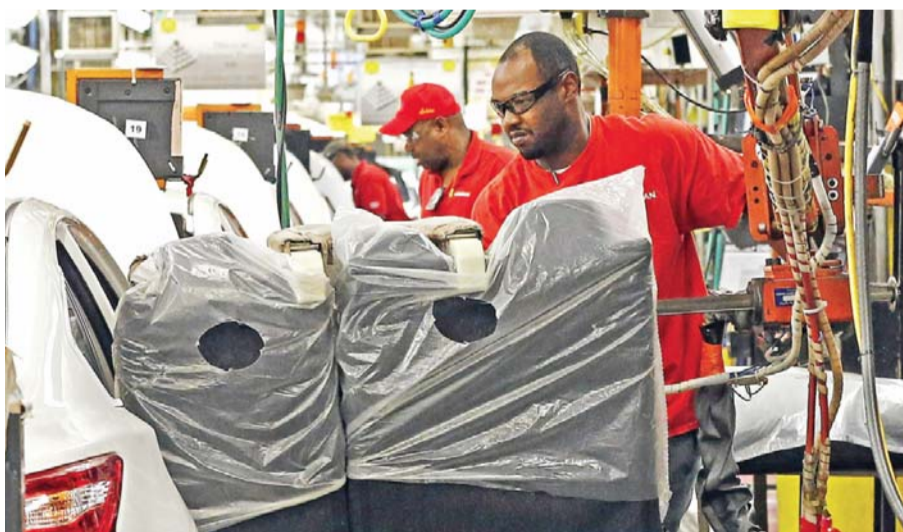
CANTON: A technician uses a lift to move a back seat section into a new Altima on the assembly line at the Nissan Canton Vehicle Assembly Plant in Canton, Miss. — AP
