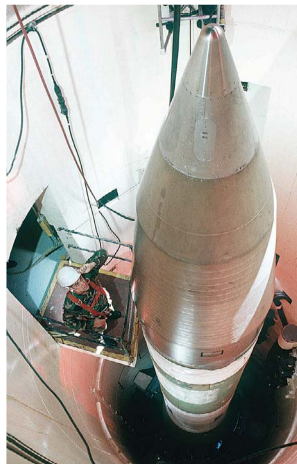
This Oct 27, 2010 US Air Force handout image shows an air force technician inspecting an LGM-30G Minuteman III missile inside a silo about 96 km from Grand Forks Air Force Base in North Dakota —AFP
