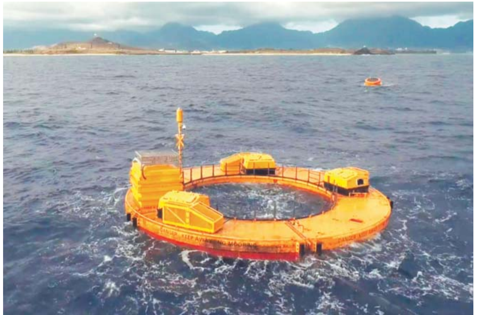
The Lifesaver wave energy device, which converts the movement of waves into electricity, is seen at the Navy's Wave Energy Test Site at the Marine Corps base at Kaneohe Bay on Oahu in Hawaii. — AP photos
