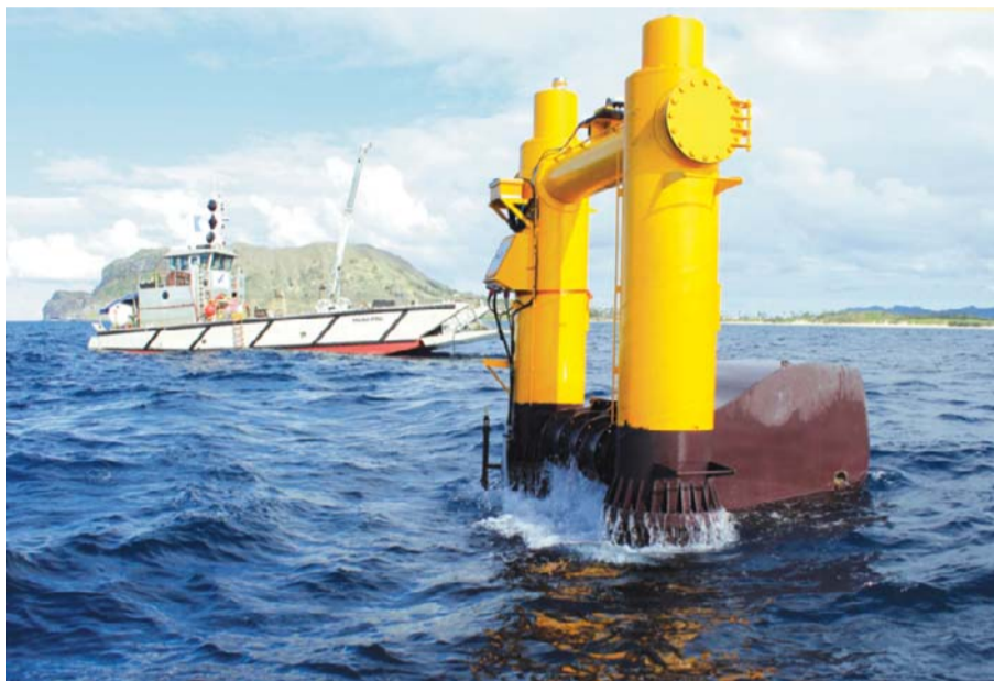
The Azura wave energy device is seen at the Navy's Wave Energy Test Site.
