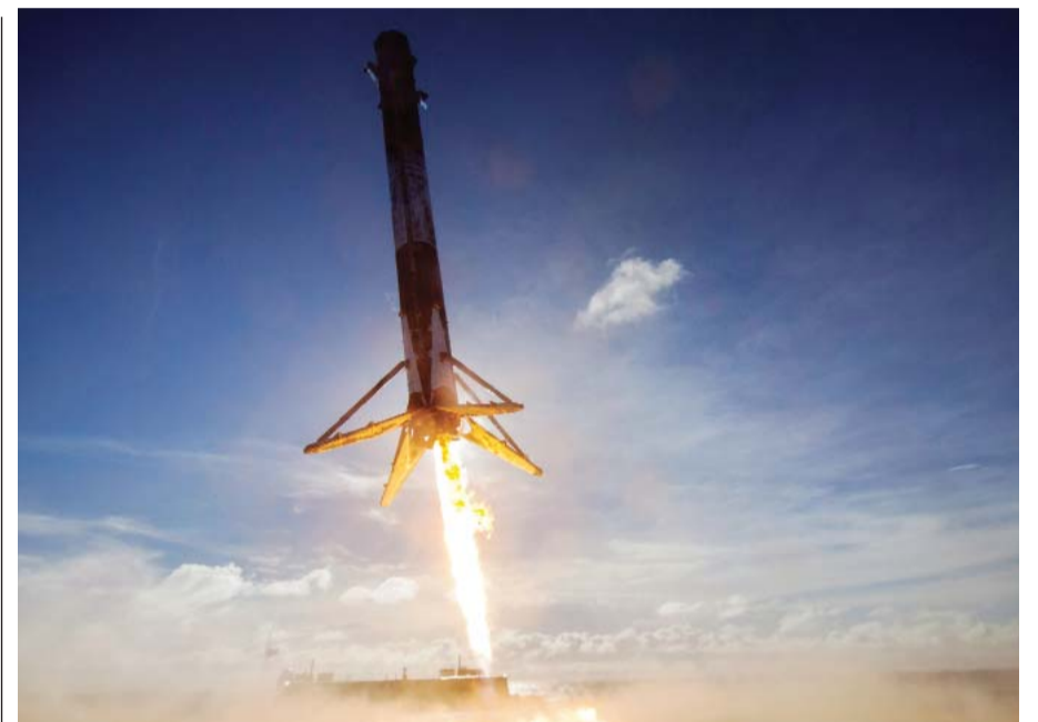
In this May 27, 2016 photo made available by SpaceX, their Falcon rocket booster lands on a platform in the Atlantic Ocean after launching a satellite into orbit. The company says it can save considerable time and money by reusing the big, expensive parts. — AP
