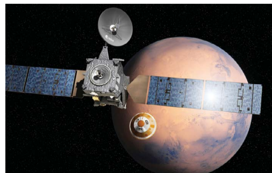
An artist's impression depicts the separation of the ExoMars 2016 entry, descent and landing demonstrator module (center) from the Trace Gas Orbiter (left) and heading for Mars. — AP
