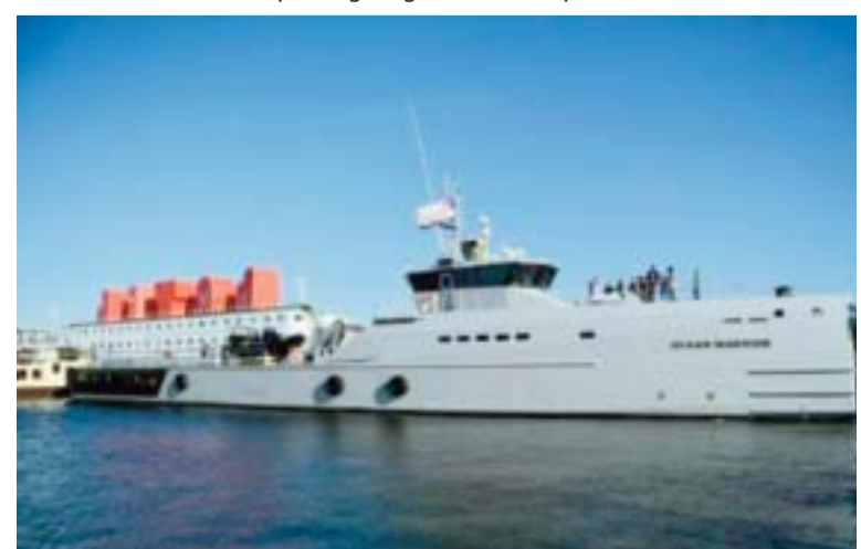
Stretching some 54 metres, Ocean Warrior is equipped with hybrid propulsion to extend its range, four powerful engines and a helicopter landing pad. — AFP
