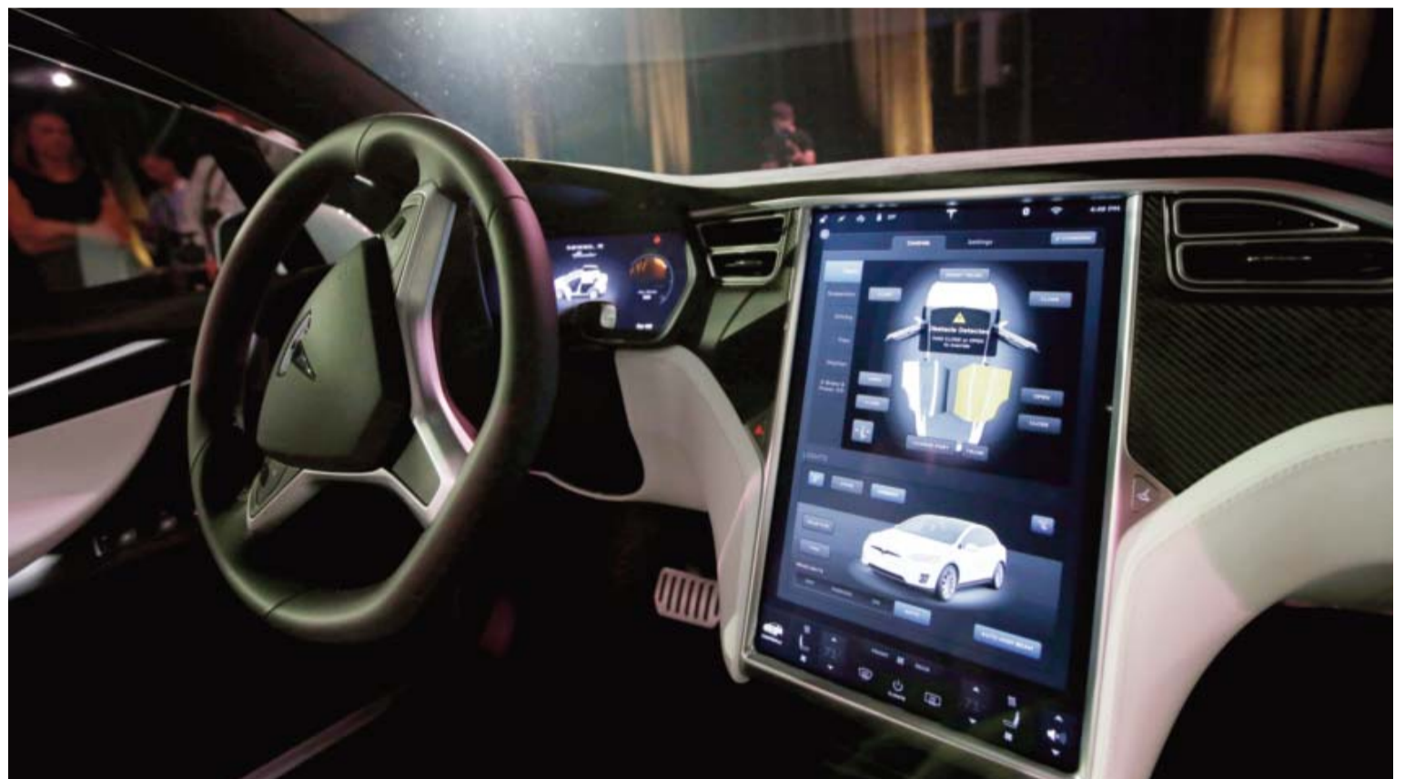
CALIFORNIA: Photo shows the dashboard of the Tesla Model X car, at the company's headquarters in Fremont, Calif. Newer cars that connect to the internet are capable of collecting vast amounts of data about their drivers. Tesla Motors has used data to reveal, sometimes within hours of a crash, how fast the driver was going and whether or not the company's semi-autonomous Autopilot system was engaged. — AP
