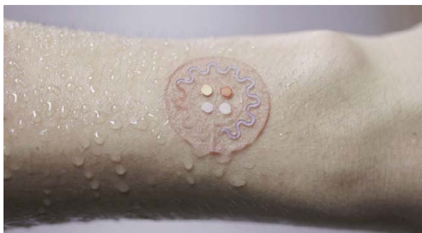
This photo shows a soft, skin-mounted microfluidic device for capture, collection and analysis of sweat. Time to break a sweat: Researchers are creating a skin patch that can test droplets of sweat to track health while people exercise, beaming results to their smartphones. —AP
