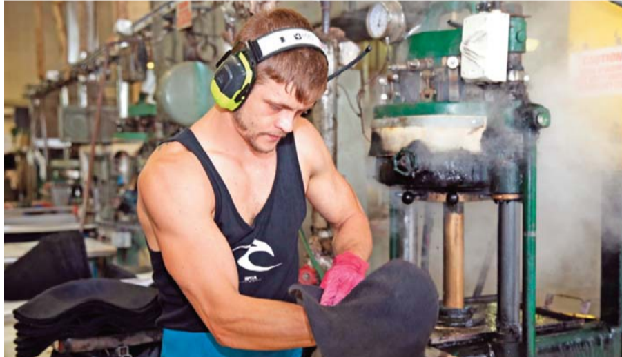
Checking for fabric floors a worker handles a hat after it is removed from a press during the hat manufacturing processes at the Akubra factory in Kempsey.
