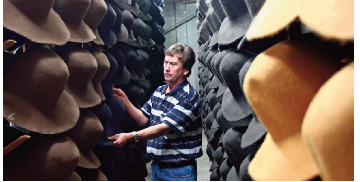
Greg Brady checks the drying progress of hats before they are sent to the final shaping department during the hat manufacturing processes.
