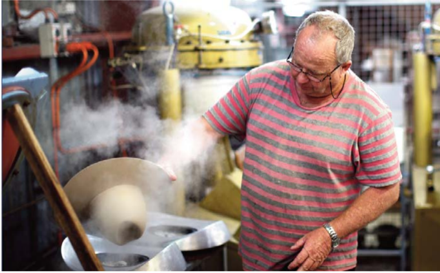
Geoff Edwards pulls a hat out of a press after the final shaping process during hat manufacturing at the Akubra factory in Kempsey, Australia.
