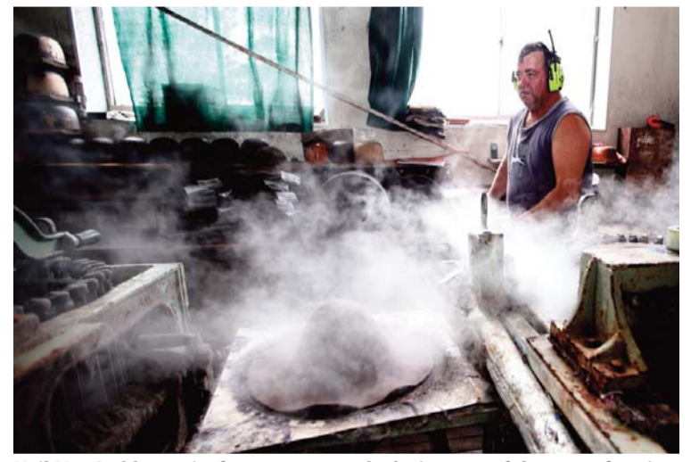
Neil MacCudden waits for steam to settle during one of the many forming stages of the hat manufacturing processes at the Akubra factory.
