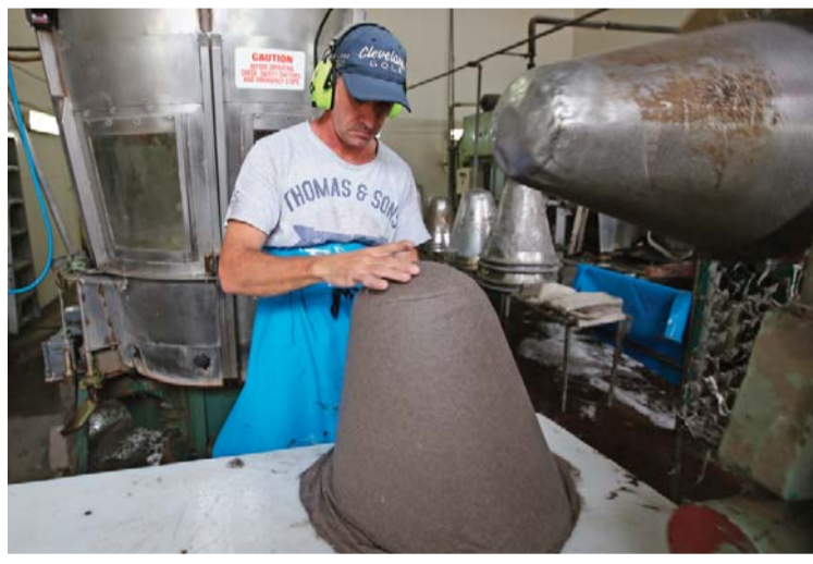
A worker in the Akubra hat factory removes a giant cone shaped form of fur felt from a stainless steel cones during the second stage of hat manufacturing.
