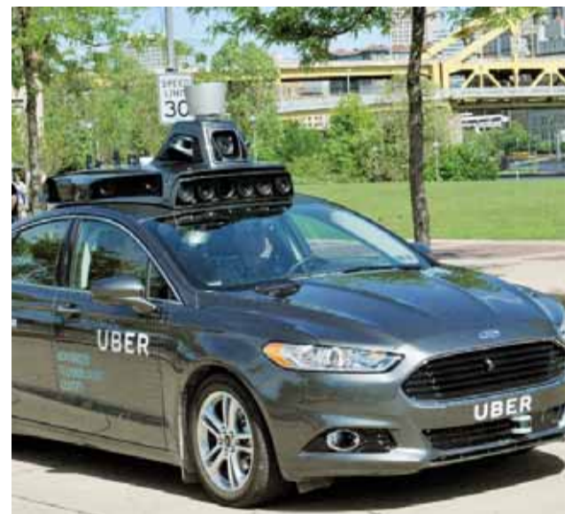
In this undated photo provided by Uber, a Ford Fusion hybrid outfitted with radars, laser scanners and high-resolution cameras drives along the streets of Pittsburgh. — AP
