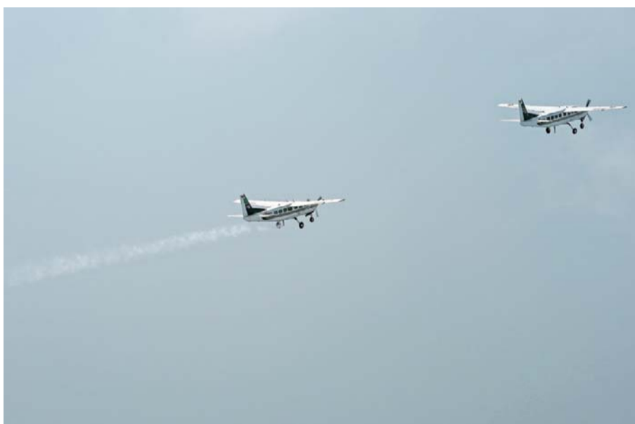
BANGKOK: (Top) Two Department of Royal Rainmaking employees depositing a sodium chloride-based material from the hold of a Cessna 208 Caravan aircraft in Nakhon Sawan to stimulate the production of rain. (Above) A pair of Cessna 208 Caravan aircraft from the Thai Department of Royal Rainmaking depositing a sodium chloride-based material above clouds in Nakhon Sawan in an effort to produce rain.
