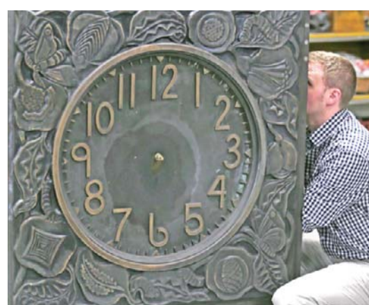
Tyler Eisner, an engineer at the Electric Time Company, works on switching the movement from gravity fed to electrically fed on a historic clock from the Silk Building in New York City.
